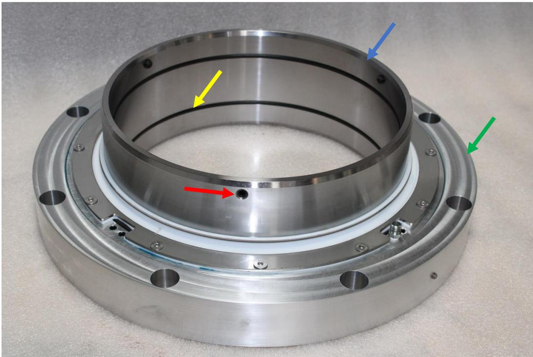
*SAPO Seal Assembly (indicated green), wear collar (indicated blue), o/ring (indicated yellow) and grub screw (indicated red)*
