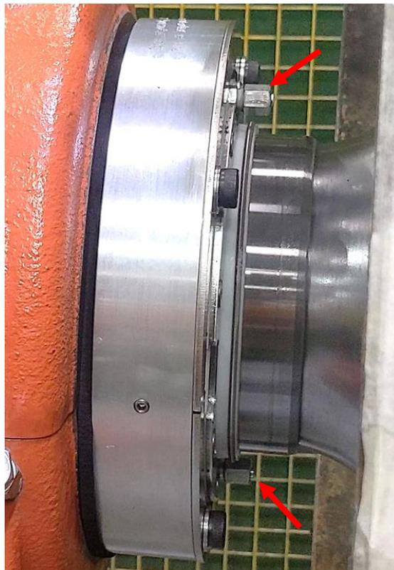
*SAPO Seal fitted with oil fittings at 12 and 6 o'clock positions on front face (indicated)*
