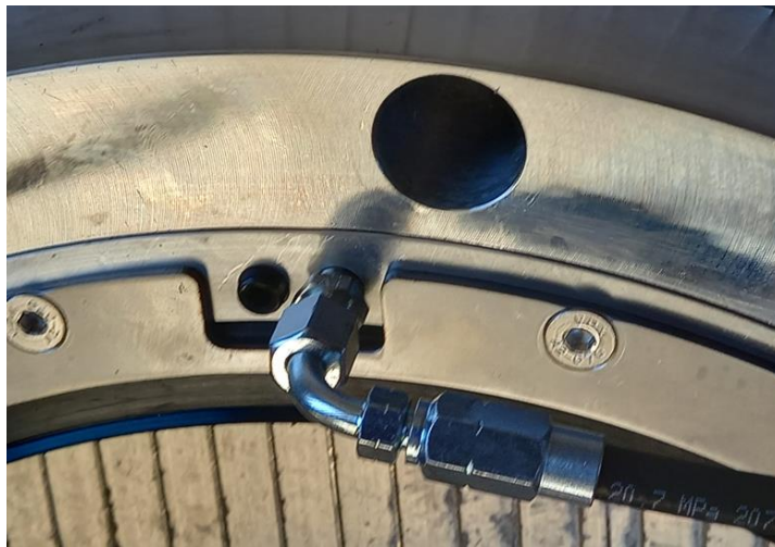
Oil line 90° std pipe end attached to SAPO seal nipple
