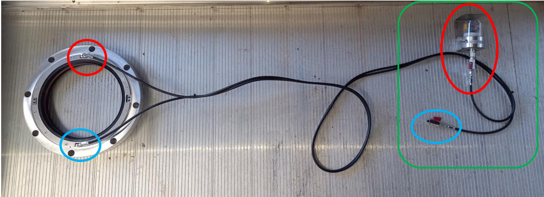
Oil system layout with inlet line attached to 12 O'clock position (ends circled red) and return line attached to 6 O'clock position (ends circled blue). Ends circled green are to be installed outside the guard within the monitoring box.
