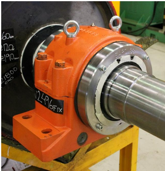
SAPO Seal installed on a drive pulley
